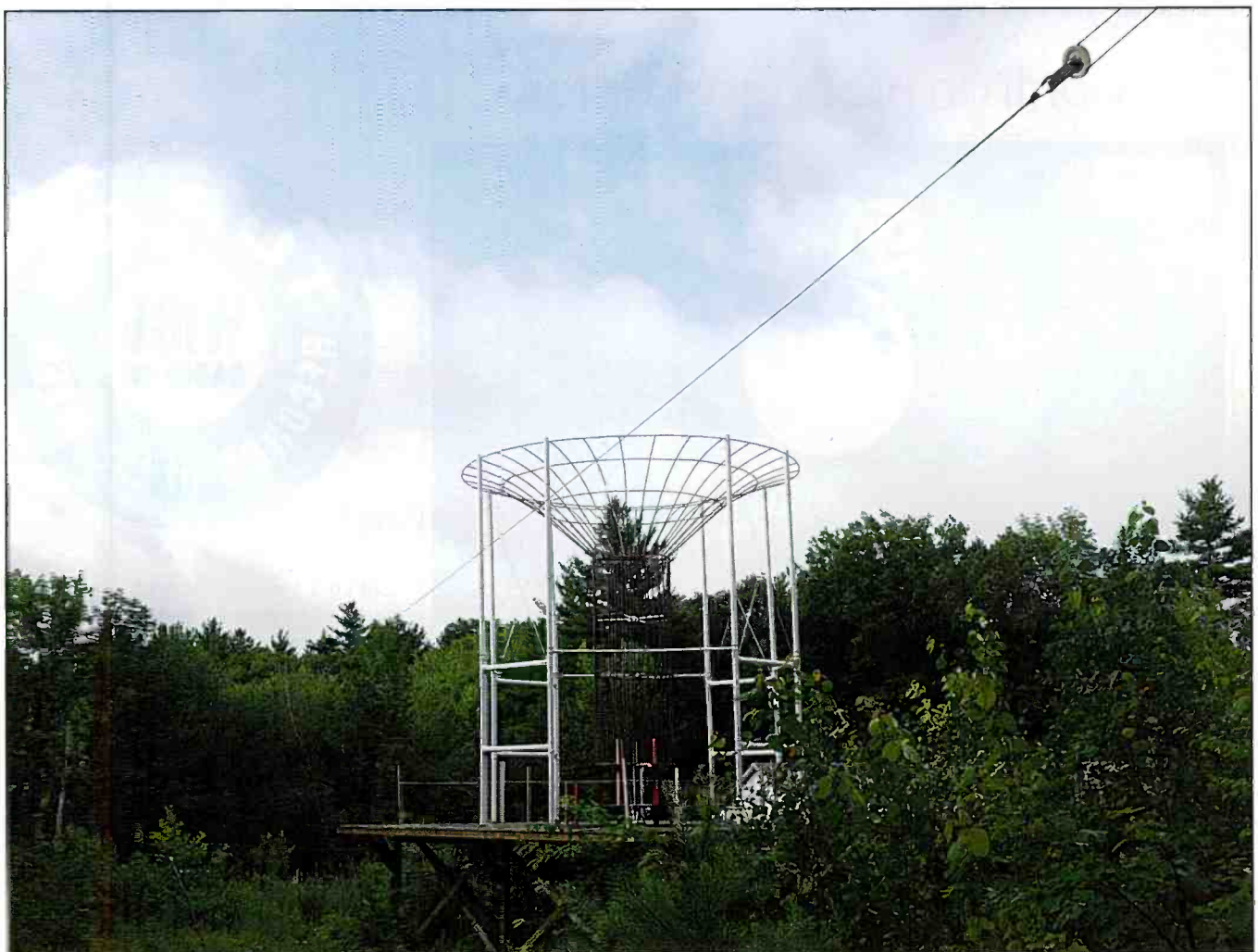
Photo C. The far end of the long wire antenna being used to transmit the signal of WGFP is visible while a CFA is under test. (WPC1CAT photo)
