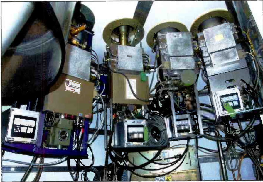
Photo G. The "loft," housing Ku, K, Q and Ka band receivers covering 12-52 GHz, is accessed via ladder.
