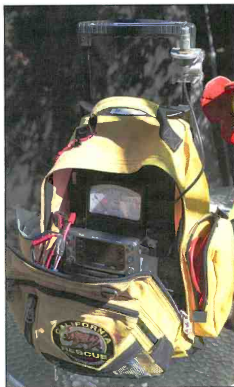
Photo G. The Emergency Communications Gordo Roller Bag is now 15 pounds lighter with the lithium-iron phosphate battery from DaySaver — offering 14-aH of run time at just 2 pounds.
