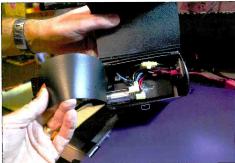
Photo E. It might be hard to imagine, but it's true: the DaySaver lithium-iron phosphate battery provides 14-aH of 12-volt DC power, yet weighs only two pounds. Wow!
