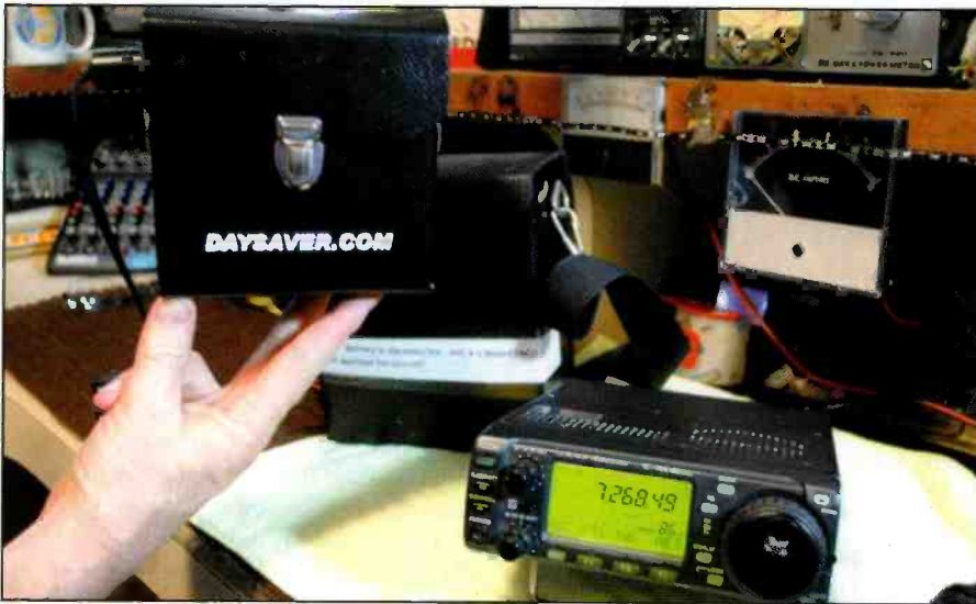
Photo C. The protective case includes circuit breakers plus a tough exterior enclosure to keep the Lithium-Iron Phosphate battery happy.
