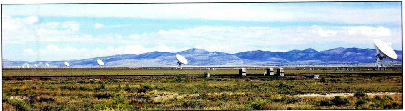
Photo L. The “A” array is extensive, using all 13 miles of the track on each of the three arms for the largest baseline for arc-second resolution.
