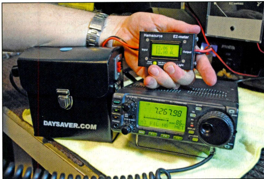
Photo A. The DaySaver Lithium-Iron Phosphate battery, shown powering this 100-watt output HF radio, gets good numbers from Gordo's monitoring volt and amp meter. ( Photography courtesy of WPC6NOA )
