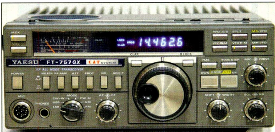
Photo F. Designed principally for radio amateurs, a Yaesu FT-757GX was used by Crossed Field Antennas Ltd., after applying for an experimental license to test CFA model MK II with 100 watts of power on 1630 kHz. (Courtesy of Universal Radio < http://www.universal-radio.com >)
