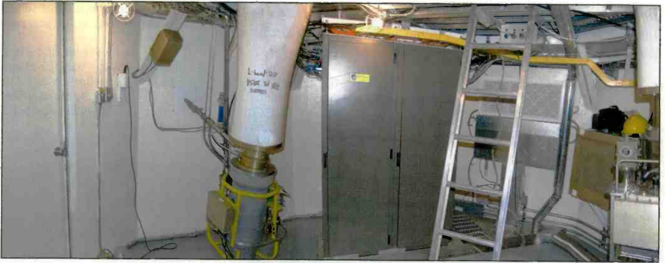
Photo E. The L-band (1-2 GHz) receiver, left, is mounted to the end of the feed horn. The LO (local oscillator) synthesizers, up/down converters, IF amplifiers, fiber optics, and so on, are in the two gray cabinets.
