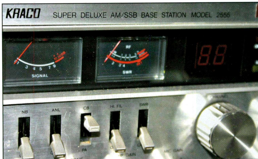
Photo A. Here's an up-close-and-personal front panel view of a classic Kraco Super Deluxe AM/SSB Base Station Model 2556 — a popular transceiver from the early days of CB SSB. (Courtesy of Wikimedia Commons)
