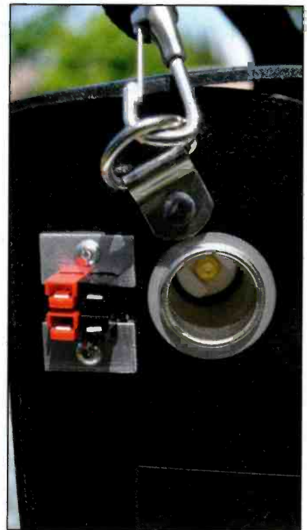
Photo D. On the side of the DaySaver pack are a pair of Anderson connectors and an accessory socket for charging of pulling current from the battery.
